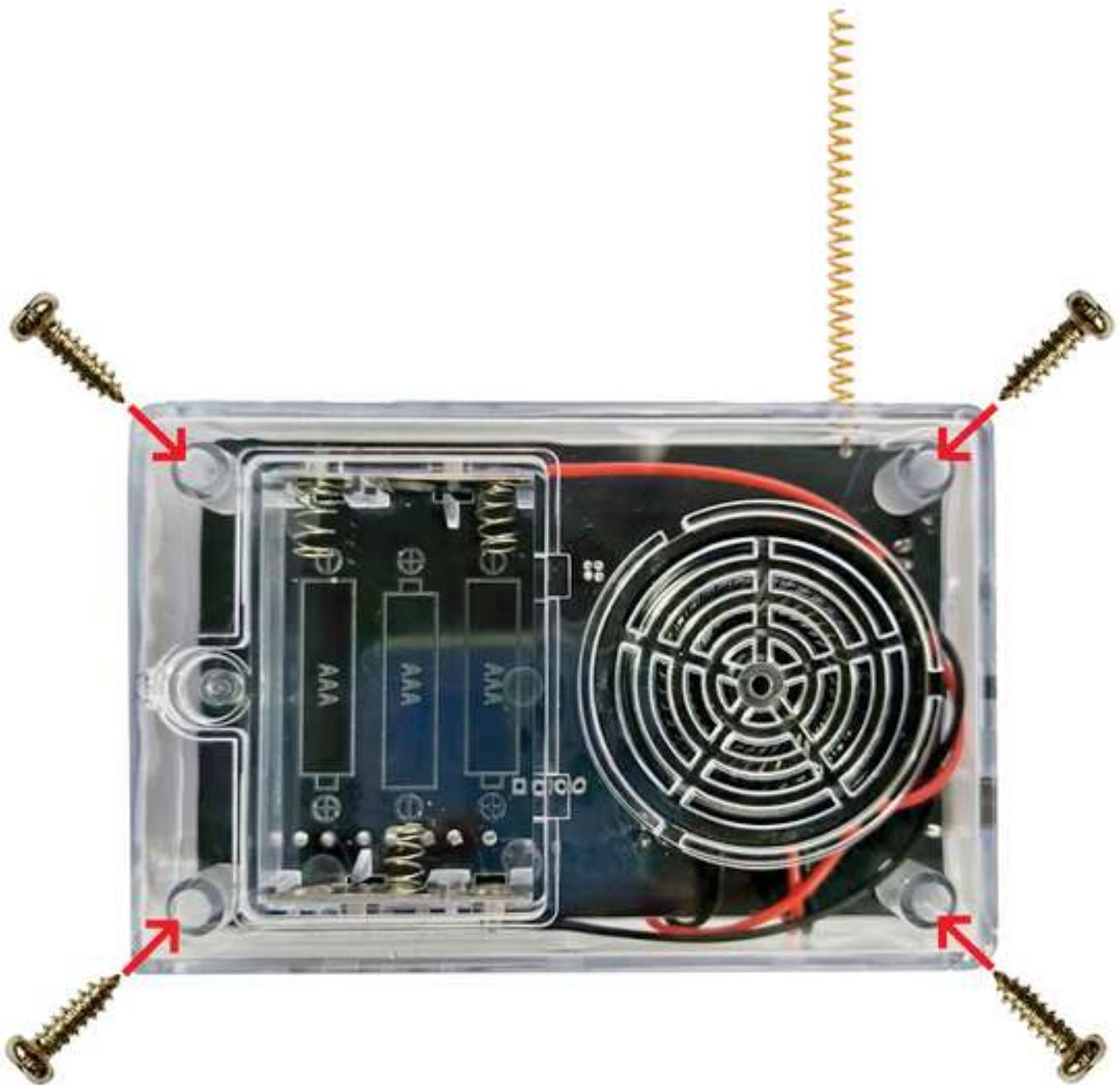
14. After installing the battery, attach the battery cover and secure it with self-tapping screw.
