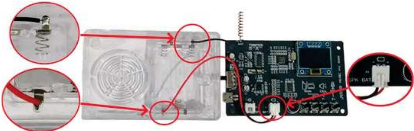
12. Weld one end of the red and black single ended terminal wire to the horn, plug the other end into the circuit board, and then insert the horn into the slot. (Red+ Black-)
