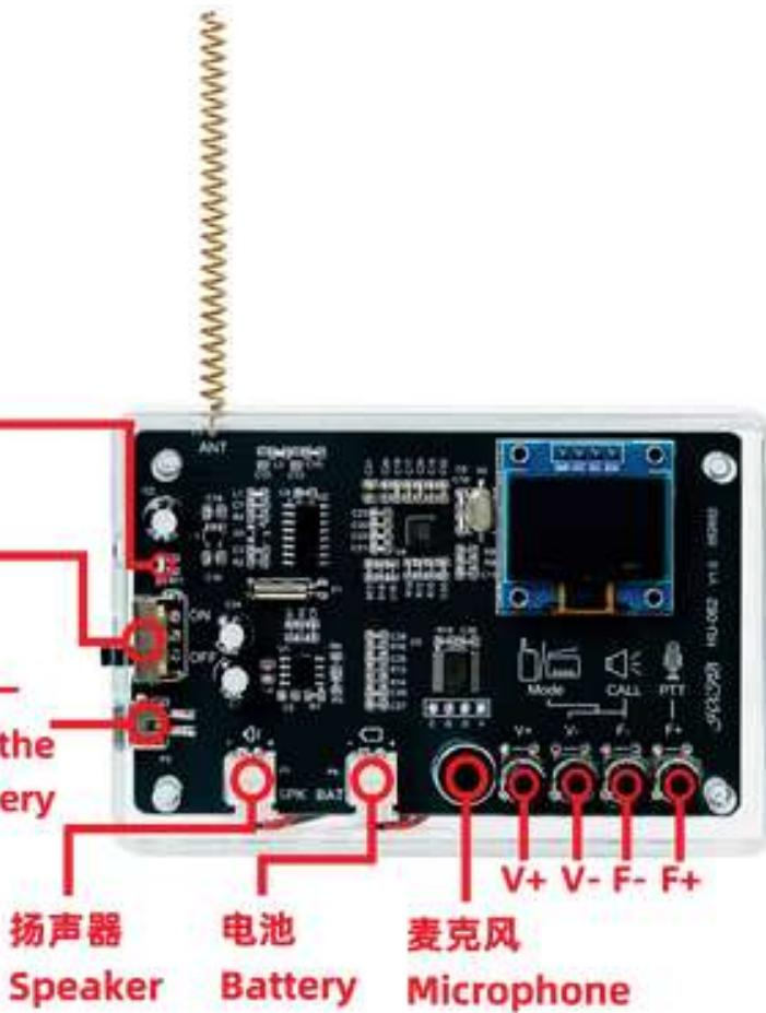
Attention: The USB interface cannot be powered on at the same time as the battery. You need to choose one or the other, otherwise the interphone may be damaged.
