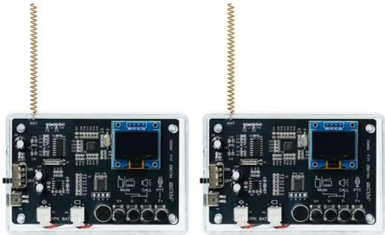
Ø Turn on the switch and in intercom mode, long press F - and F+ to enter crystal oscillator deviation compensation mode
