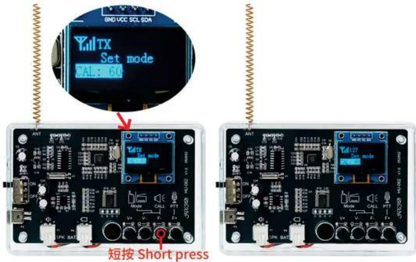
Ø Adjust the compensation value through V+ or V - until a stable RX icon is displayed in the upper right corner of the receiving mode walkie talkie
